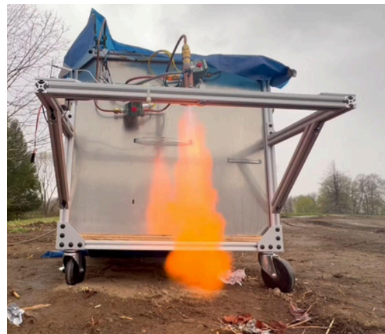
The team with our gaseous oxygen/isopropyl alcohol copper torch igniter from last semester
