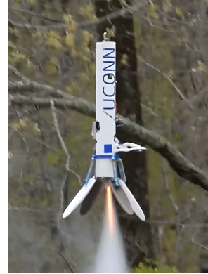
Apr. 30, 2023. Successful stabilization during drop test.
